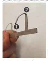
Bend the tip slightly **1**, bend in the middle as shown **2**
